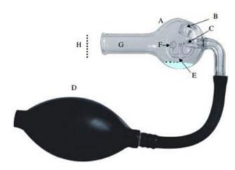
The Nebulizer is a small device that atomizes small aqueous volumes in order to effectively distribute particulates and suspensions, for example, for thorough analysis. Throughout work in Electron Microscopy, grids are held vertically in relation to the Nebulizer outlet. A flexible bulb (D) is squeezed to release a direct spray. The unique all-glass design is perfect for easy, yet thorough cleaning, ready-to-use for all application.
